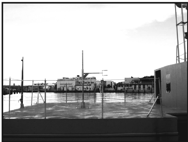
Fig. 1 Patrol craft YP 676, with a modified flight deck and aft hangar-like superstructure.
